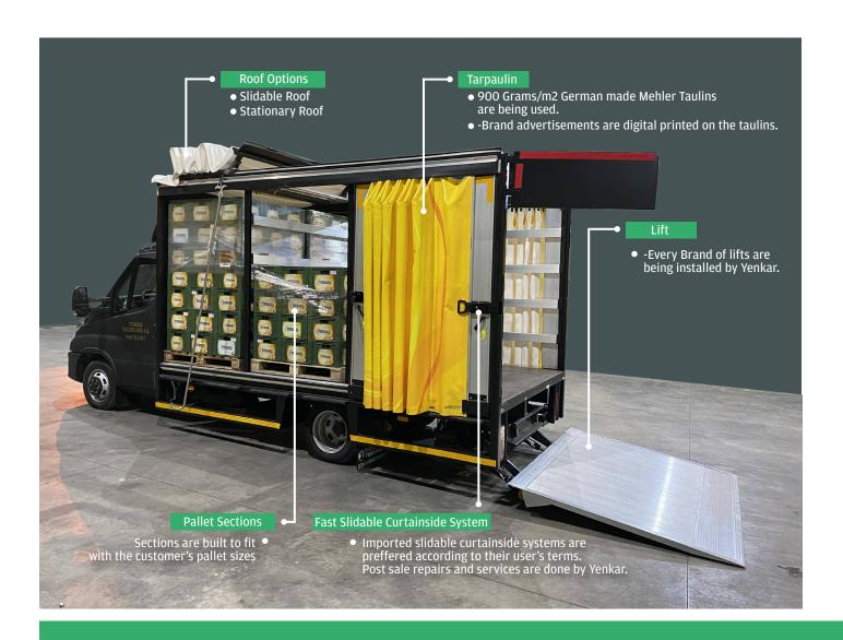
Slidable Curtainsider system has to work well, therefore it is secured with a side barrier profile and plastic chocks, preventing the forklifts to harm the slidable system rails. This product has many options that can be added to it with customer demand.
